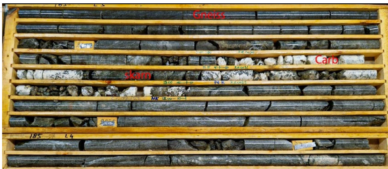
Figure 9. 10m of core with two carbonatite dikes with skarn on either side of the calcite carbonatites. Importantly these units are easily discerned/geologically modelled and well logged in the past in the case of historic core.
