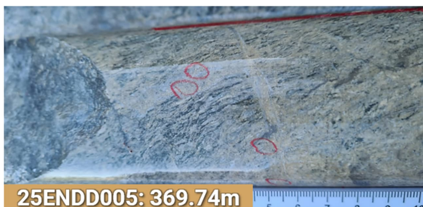
Photo 1. Visible gold (circled red) in hole 25ENDD005 in various places within 345.98-369.74m down hole in Fe-Carbonate quartz-pyrite-arsenian pyrite \pm adularia veins within granite host rock.
