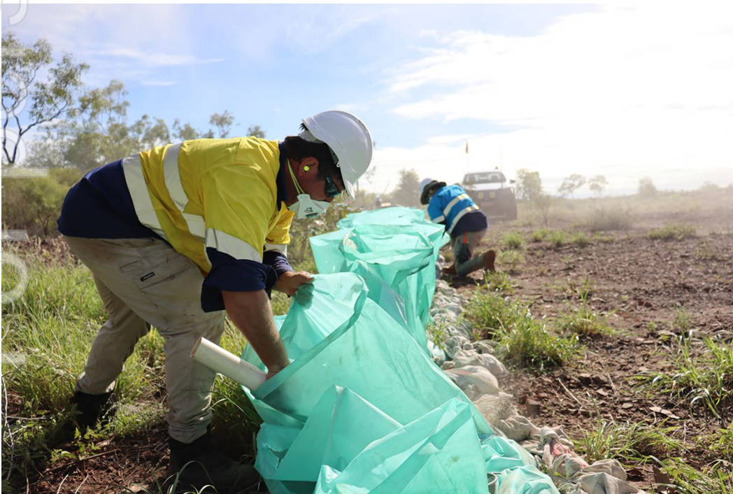
Photo 2. Spearing sample with PVC for the geological chip logging (GAM drill program).
