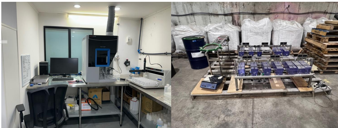
Figure 2 (L). ICP analytical machine capable of reading up to 66 elements to ppb levels of detection.
