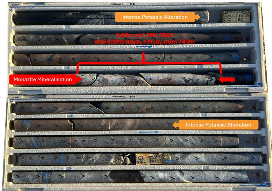
Figure 2: MWDD01 structurally controlled carbonatite dyke, 0.85m at 1.39% TREO and 0.20% Nd_2O_3 + Pr_6O_{11} from 74.1m within intense potassic alteration halo. The mineralisation represents a new REE mineralisation lode not observed at surface.
