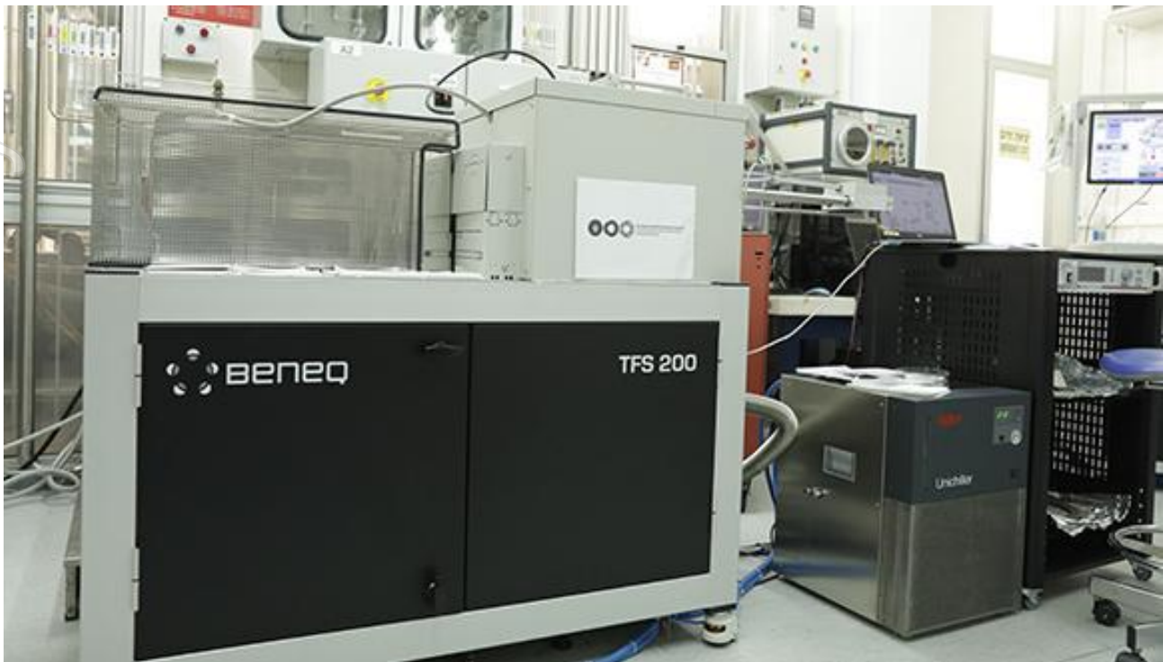
Figure 1: the Beneq TFS 200 ALD system at the Tel Aviv University's Jan Koum Center for Nanoscience and Nanotechnology
