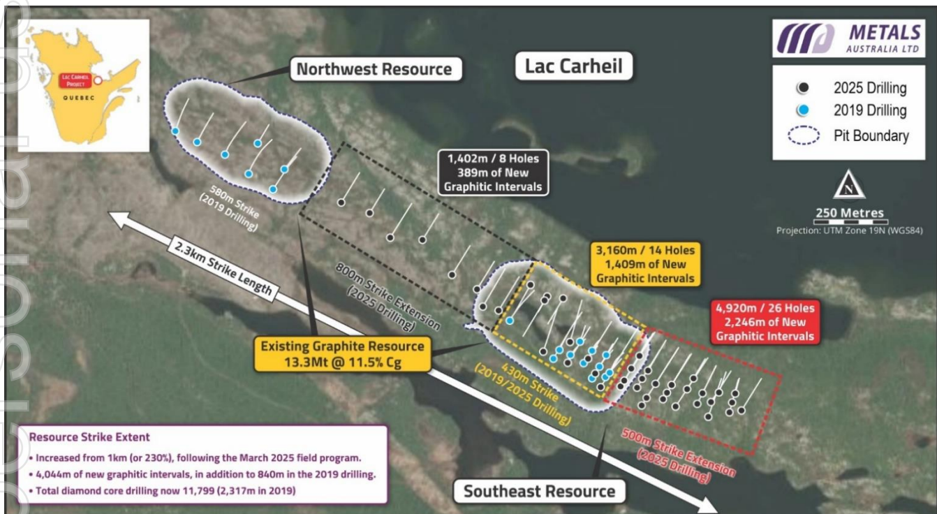
Figure 1 - Lac Carheil Graphite Project – Existing Mineral Resource zones and drill holes (blue collars) and new drilling zones and drill holes (black collars). Zone meters drilled, graphite intervals logged, and strike length are also noted.
