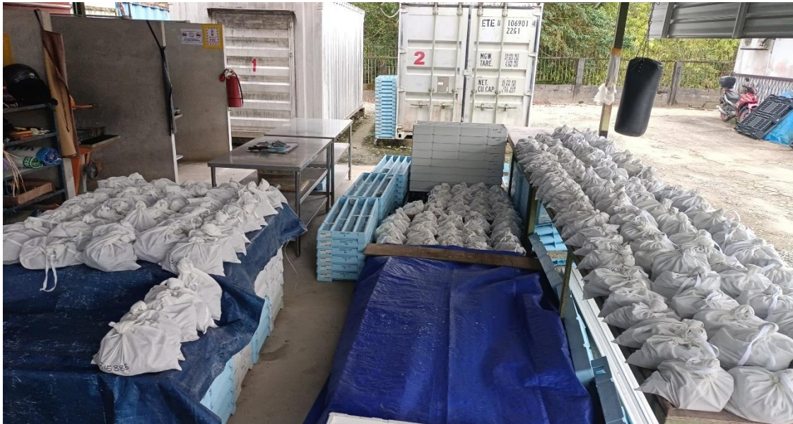
Figure 5 – Approximately 700 kg of core samples from JUDDH-127 bagged and ready for despatch to ALS for storage and specialist testing.
