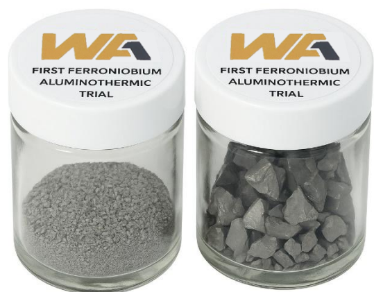
Figure 5: WA1 proof-of-concept testwork ferroniobium fines & lumps
