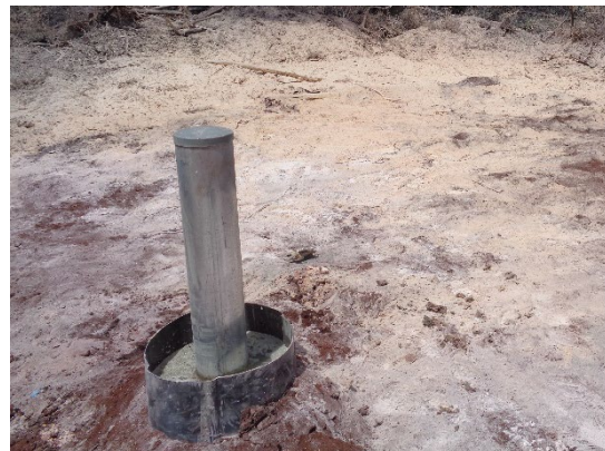
(left) drill cores from the geotechnical drilling campaign (right) groundwater monitoring bore installed at the Toondoon mine site
