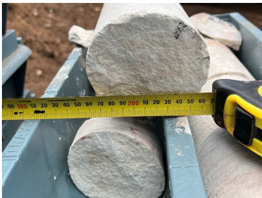
(left) drill cores from the geotechnical drilling campaign (right) groundwater monitoring bore installed at the Toondoon mine site
