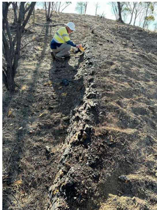
Figure 13. Base Metal Target - Outcropping fine-grained sedimentary rock of the Ronlow Beds with cleavage steeply dipping toward NE - strike NW-SE - yellow-ochre, black & brown limonite possibly derived oxidation of sulphides at depth. The petrology sample collected at this location (GDA2020 343440mE and 7483340mN Zone 55) and shown in Figure 11.
