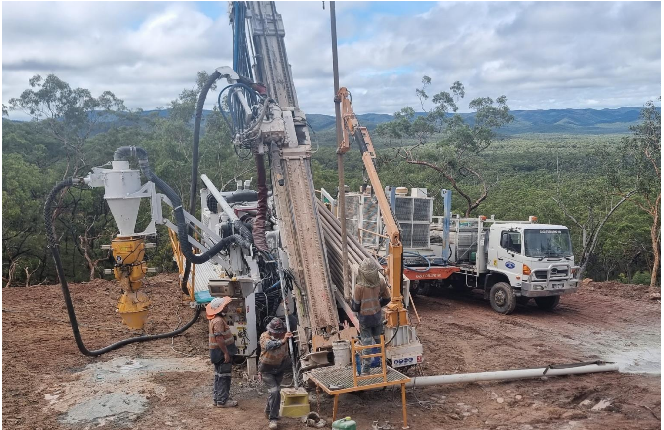
Figure 4 Track-mounted reverse circulation (RC) drill rig at Orient West (ORR069)
