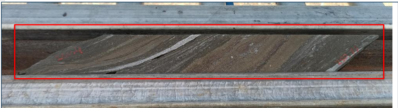
Figure 9: Photo of diamond drill core from GLPDD009 (250.40-250.77m) showing massive to semi-massive sulphide lode with banded pyrite (yellow), sphalerite (red), galena and chalcopyrite. The associated sample interval GRD11404 (250.15-251.15m) returned 5.49g/t AuEq.
