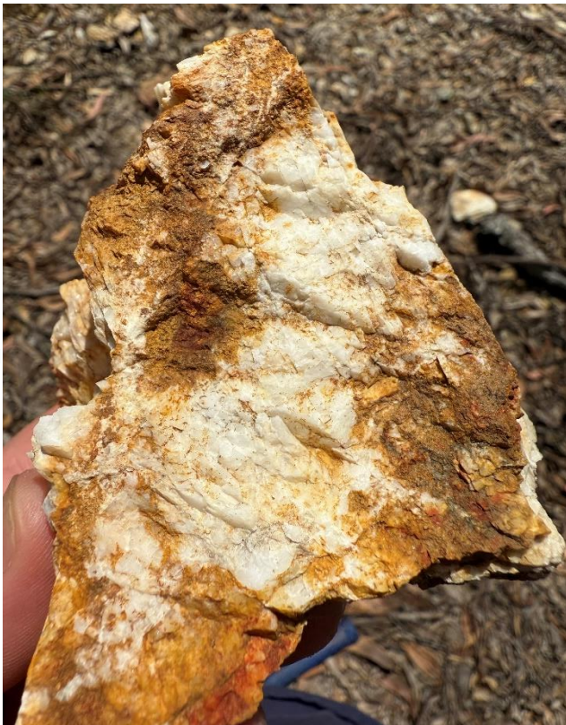
Figure 14 – Gold mineralisation within ferruginous rusty quartz vein yielding 63.10g/t Au from sample 3001227
