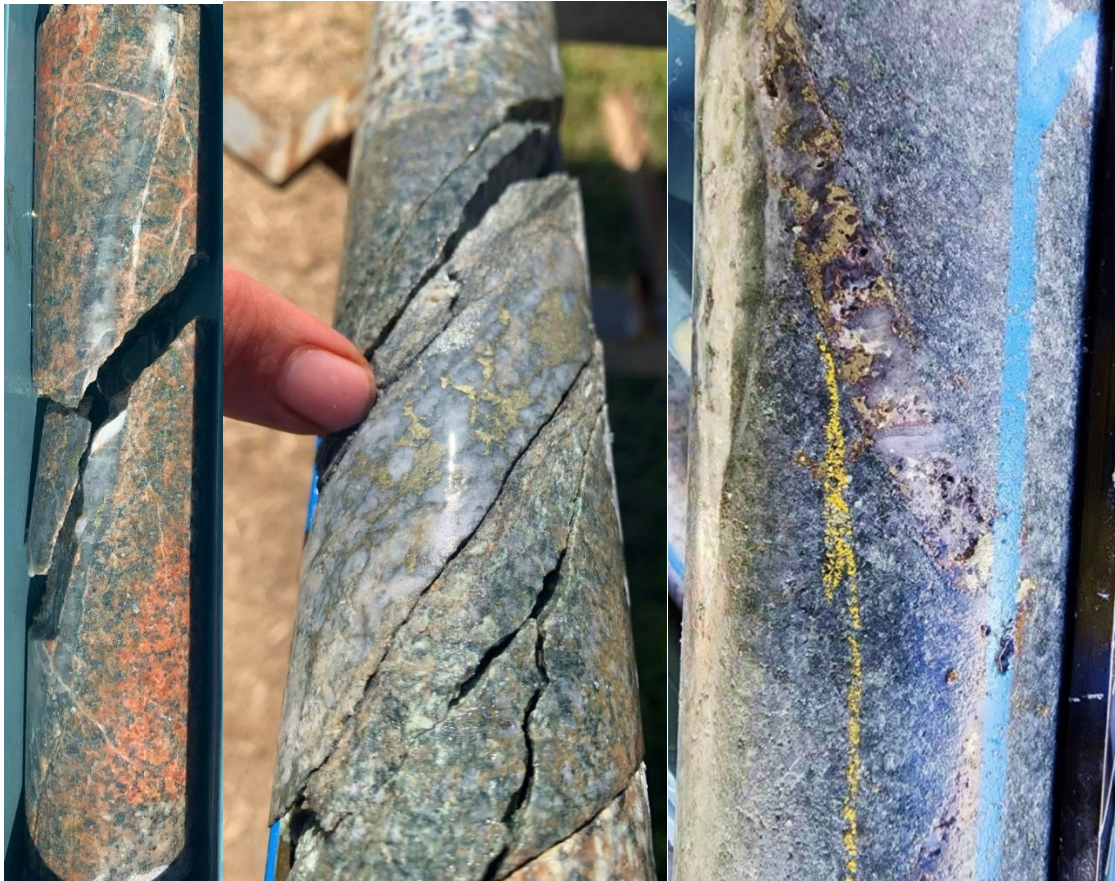
Figure 4. Left to Right. MRDD001, 227.3m strong potassic alteration of granodiorite with sulphide bearing quartz-vein (0.6m @ 10ppb Au, 0.5g/t Ag & 857ppm Cu). MRDD002, 136.15m quartz-sulphide vein within shear of strong sericite alteration of granodiorite (0.5m @ 9.35g/t Au, 21.1g/t Ag & 0.7% Cu). MRDD003, 34.9m strong silica and sericite alteration in granodiorite, quartz veins with visible chalcopyrite (0.6m @ 0.3g/t Au, 37g/t Ag & 1.6% Cu). (ASX announcement 21 October 2024)
