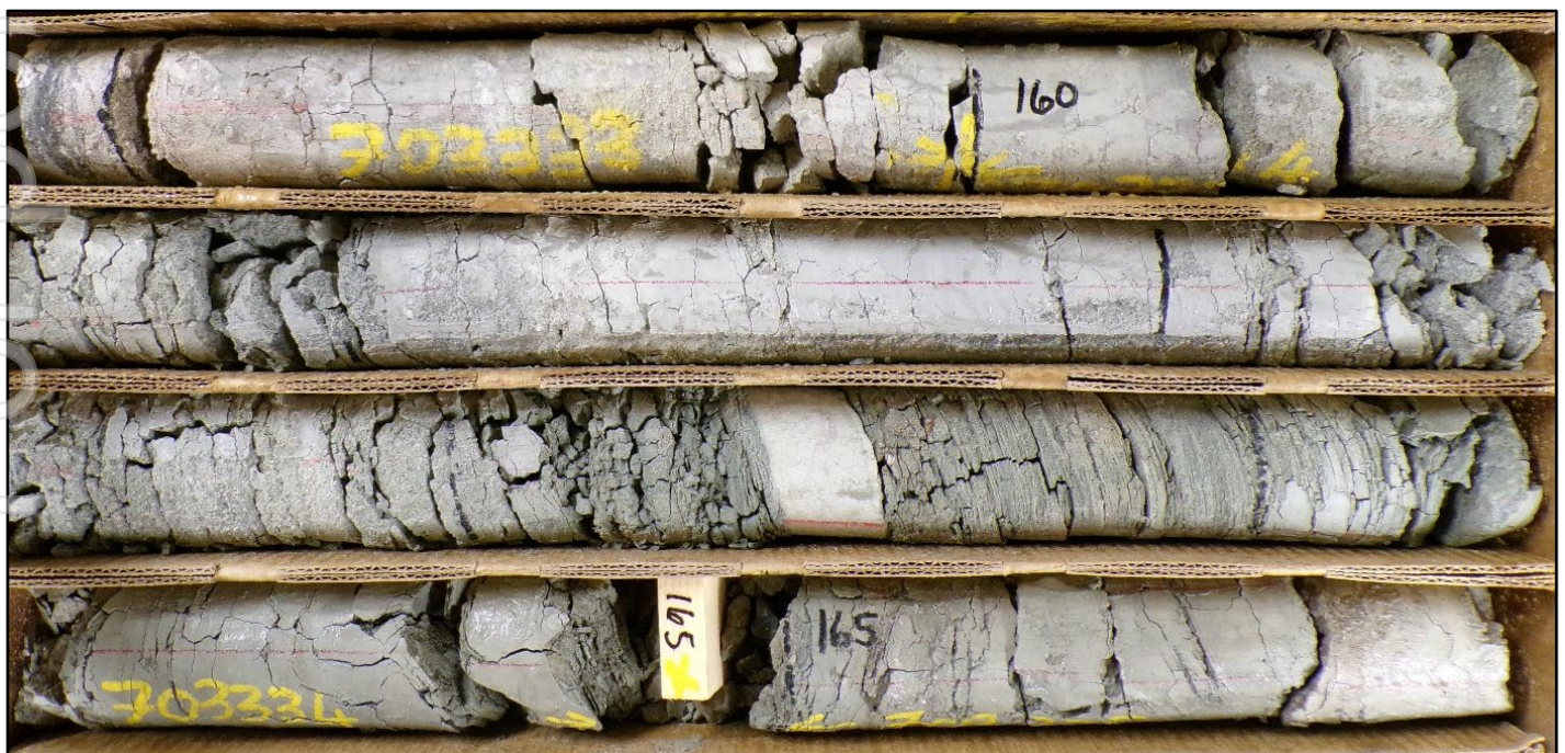
Figure 3. High-grade clay rich RMDD002 drill-core from 48.8-50.3m (160-165ft) which assayed 3,280ppm Li.
