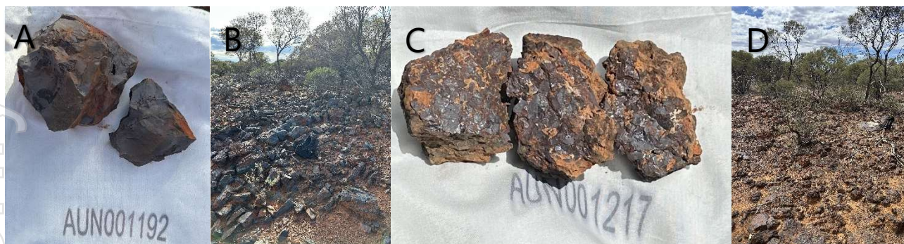
Figure 15. (A) Hematite enriched BID (Sample AUN001192 – 65.17% Fe), (B) outcropping hematite enriched BID, (C) hematite enriched capping / pisolite (Sample AUN001217 – 59.62% Fe), (D) outcropping cemented hematite pisolite potentially representing immature paleochannel iron deposits or capping.
