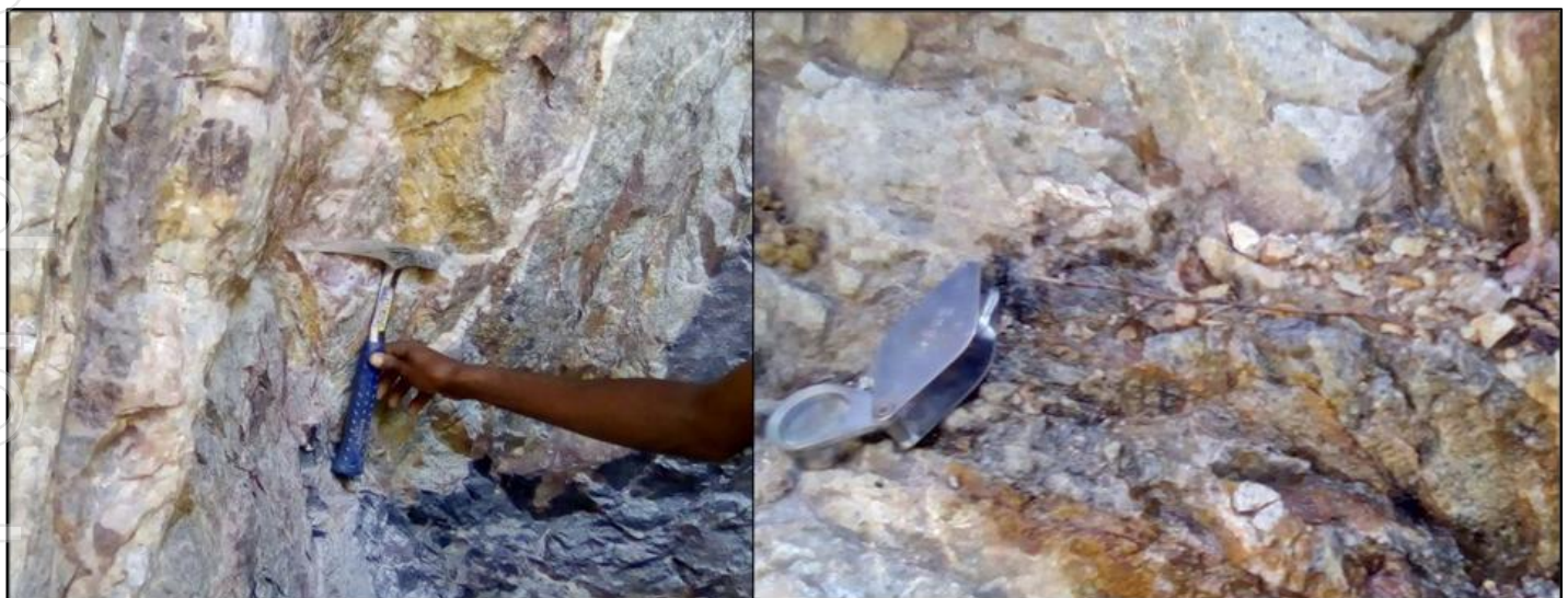
Figure 5: An exposure of an artisanal mining pit at the Lega Dembi South Project showing deformed white quartz veins along with intensive wall rock alteration.
