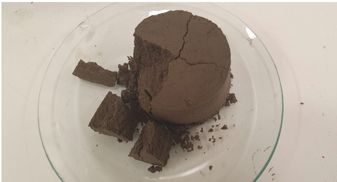
Dry-stackable tailings filter cake produced using Clean TeQ's ATA® technology with vacuum filtration
