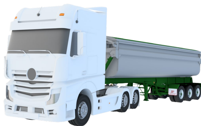
Figure 2. Conceptual Render of bespoke, lightweight, enclosed side tipping semi-trailer for coal transportation.
