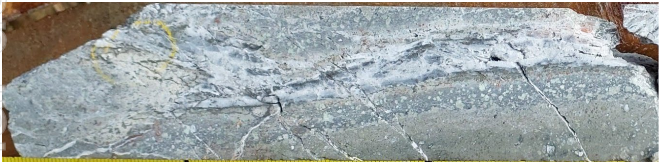
25VDD002_195.76-196.15m. From Sample No. 386651, 195.76-196.56m (0.8m) 11.4 g/t Au, 6.52 g/t Ag. Mineralised chalcedonic vein within strong clay-altered basalt. Colloform and crustiform epithermal vein textures, open spaces with drizzly quartz. Blebby and disseminated pyrite, sphalerite and grey sulphide.
