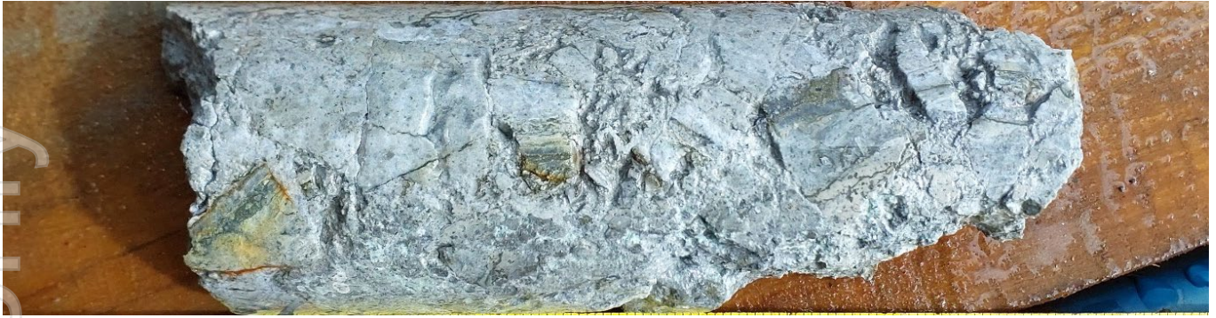
25VDD002. 185.88_186.02m. From Sample No. 386641 – 185.34-186.23m (0.89m), 0.95 g/t Au, 5.33 g/t Ag. Clasts of mineralised chalcedonic vein with rock flour and mineralised silicified-cemented matrix. Clasts display fine sulphidic breccias with pyrite-dark sulphide. Disseminated, blebby and wisps of pyrite-sulphide in brecciated-milled clay-altered basalt, tuff or andesitic dyke.
