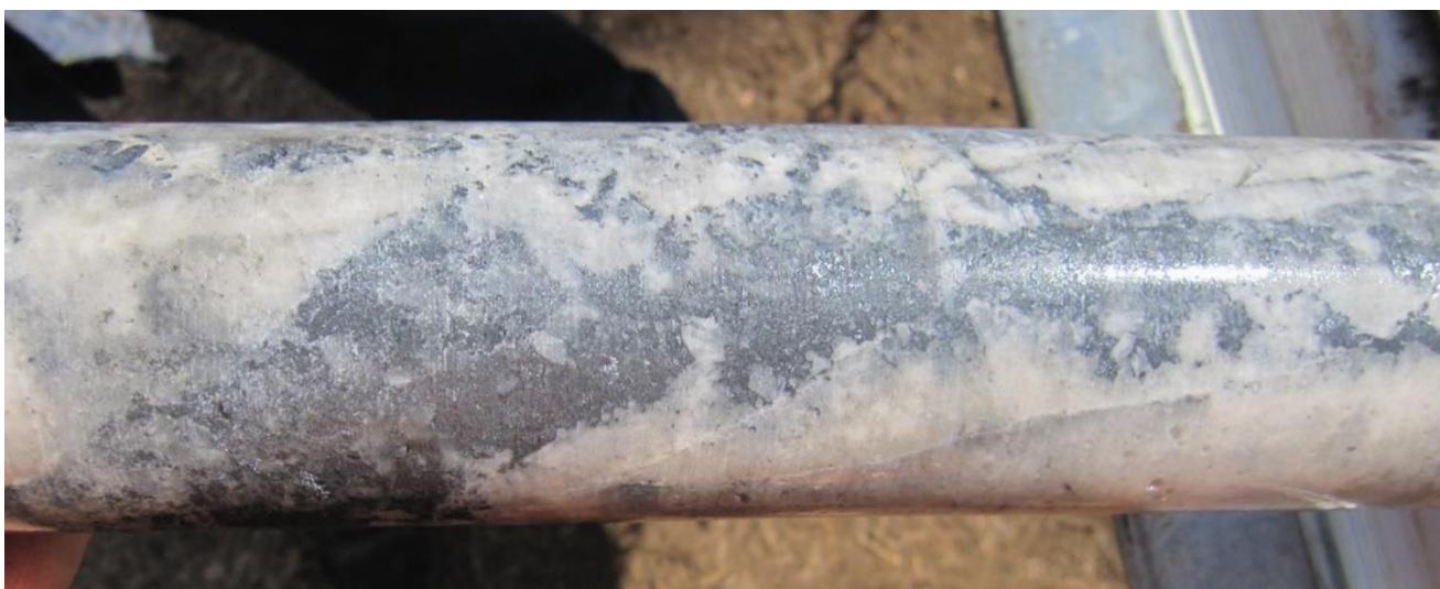
Figure 10: The Banshee core pictured, drill hole CNDD01 89.9m-90.2m, was part of a zone that assayed 1.25m @ 5.23% Sb and 1.39g/t Au (ASX: GDM Prospectus 2023 and ASX: GDM Sep 2024 ).
