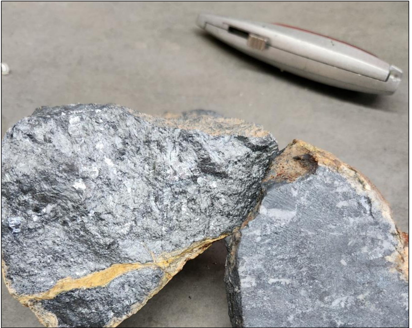
Figure 11: High-grade stibnite from Banshee antimony mine waste dumps (not In-situ). Broken rock face on the left, sawn rock face on the right. No samples taken or submitted for analysis.
