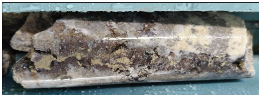
Figure 5: Sulphide Vein from TRDD001A (HQ core size) showing sulphides within quartz and carbonate veining, included in sampling from 77.1 to 77.6m (ASX: DTM Mar 2025)
