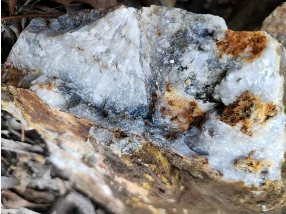
Figure 8: Sulphides in quartz from sample DRC006, abundant pyrite and arsenopyrite. Small quantities of stibnite (0.2%) was tentatively identified and is subject to confirmation by assay.
