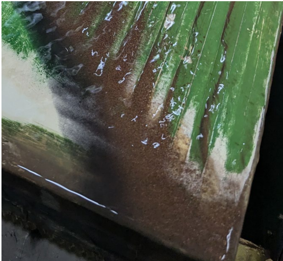
Figure 5: Shaking table test work distinct mineral banding highlights excellent gravity separation potential of the Mata da Corda ore.
