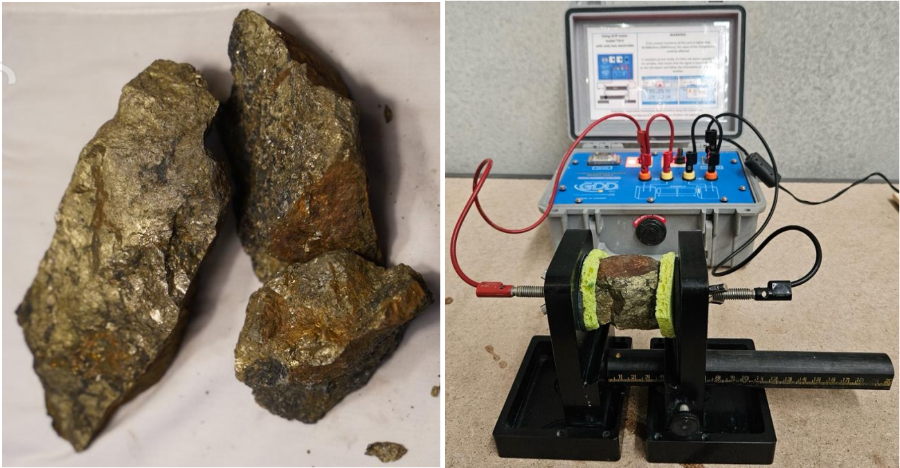
Figure 10: Prince Of Wales prospect sample RK008302 10.15% Cu and 65.8g/t Ag 11 , being tested for Induced Polarisation, chargeability, galvanic resistivity and inductive conductivity
