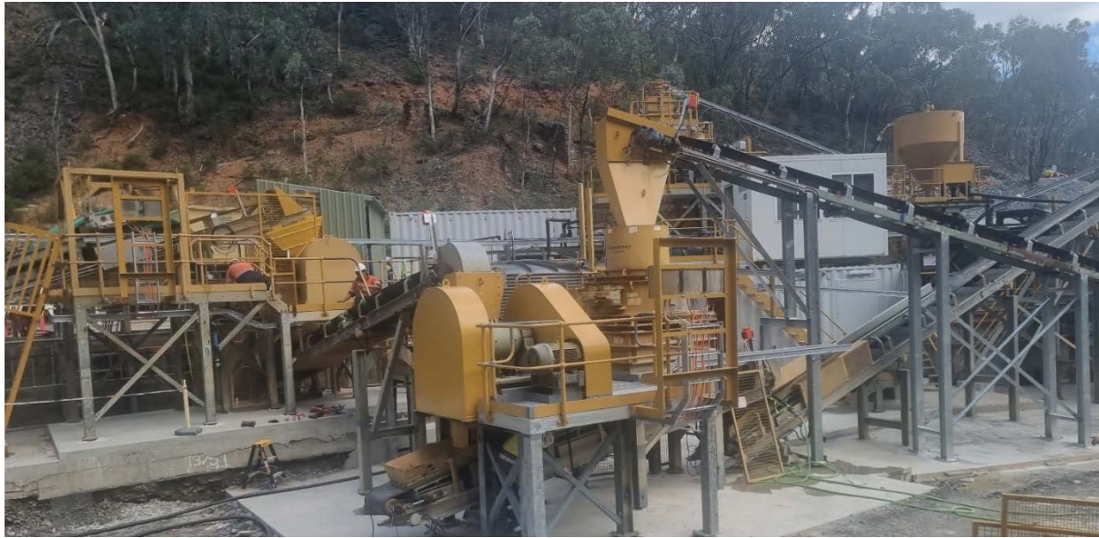
Figure 13: Reward gravity gold plant looking over the 2 jaw crushers and the impact crusher
