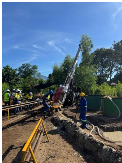
Figure 2 Diamond drill rig in operation
