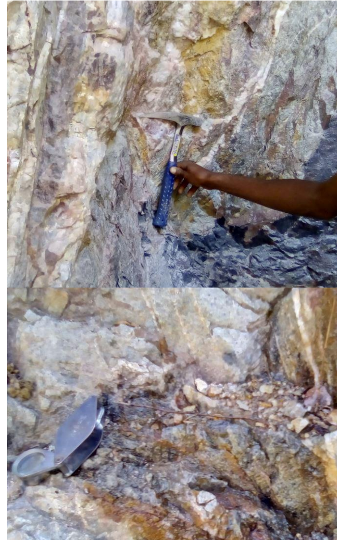
Images: An exposure of an artisanal mining pit at the Lega Dembi South Project showing deformed white quartz veins along with intensive wall rock alteration
