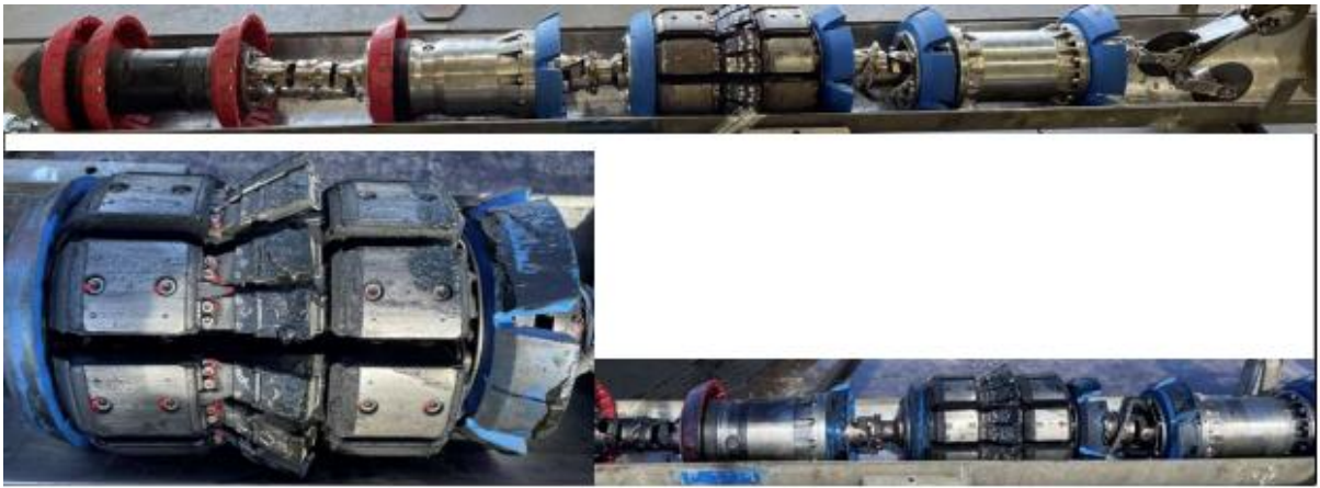
Photo of the Intelligent Pig that was run inside Cliff Head Oil Production and Water Injection Pipelines
