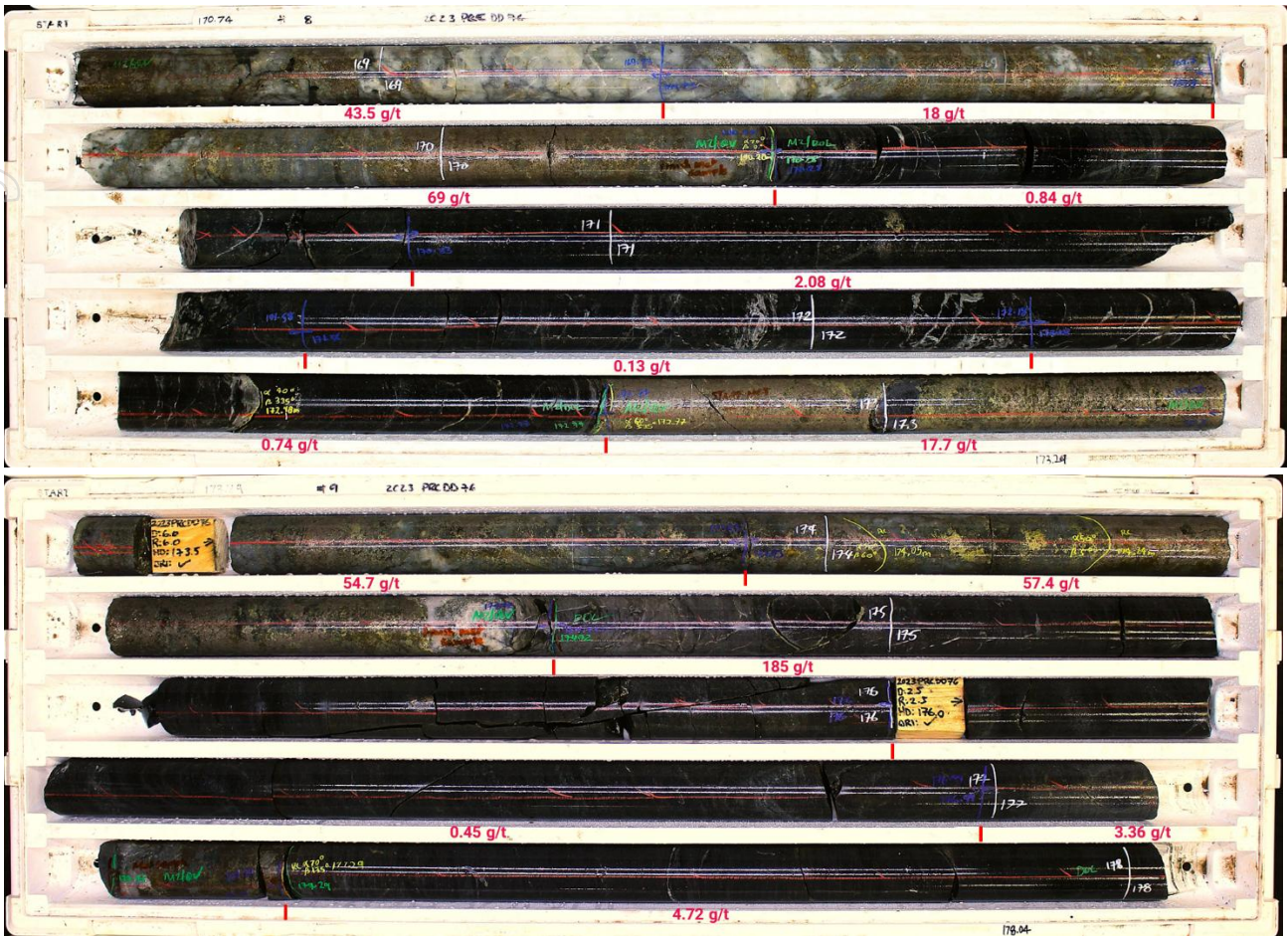
Figure 4: 35m @ 14.12 g/t Au diamond drill core from hole 23PRCDD076 showing Paris-style gold mineralisation as massive sulphide assemblage including pyrrhotite and chalcopyrite with structurally controlled quartz veins. Refer to ASX Announcement 5 July 2023.
