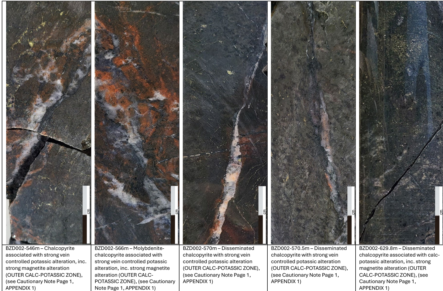
Figure 4: Core photos from Breccia West diamond drilling (see Cautionary Note Page 1, APPENDIX 1)
