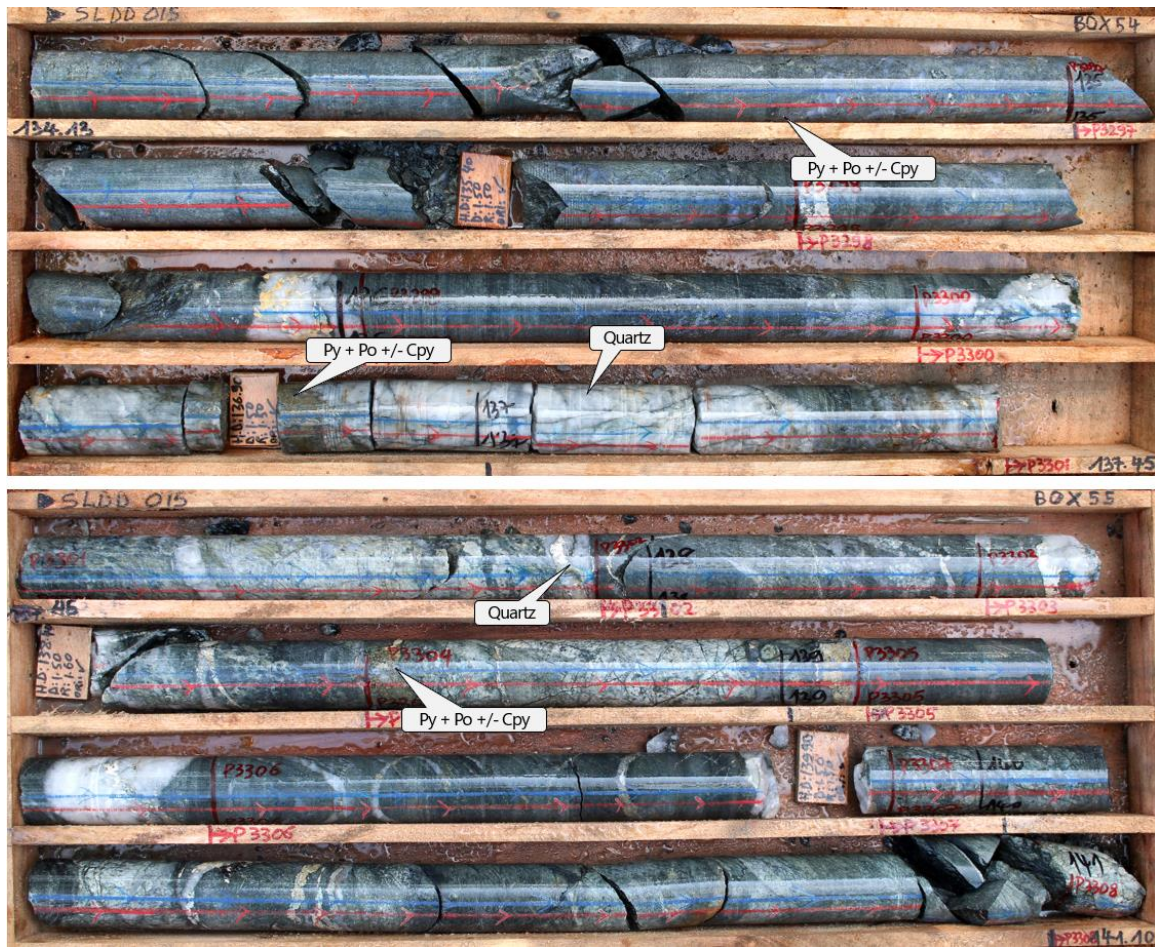
Figure 9: Veining and sulphides in hole SLDD015 showing quartz veining (~30%) associated with pyrite (Py - 1 to 10%), pyrrhotite (Po - trace to 3%) and chalcocopyrite (Cpy - trace to 1%) seen from 135.6m to 141.4m (refer Table 2).
