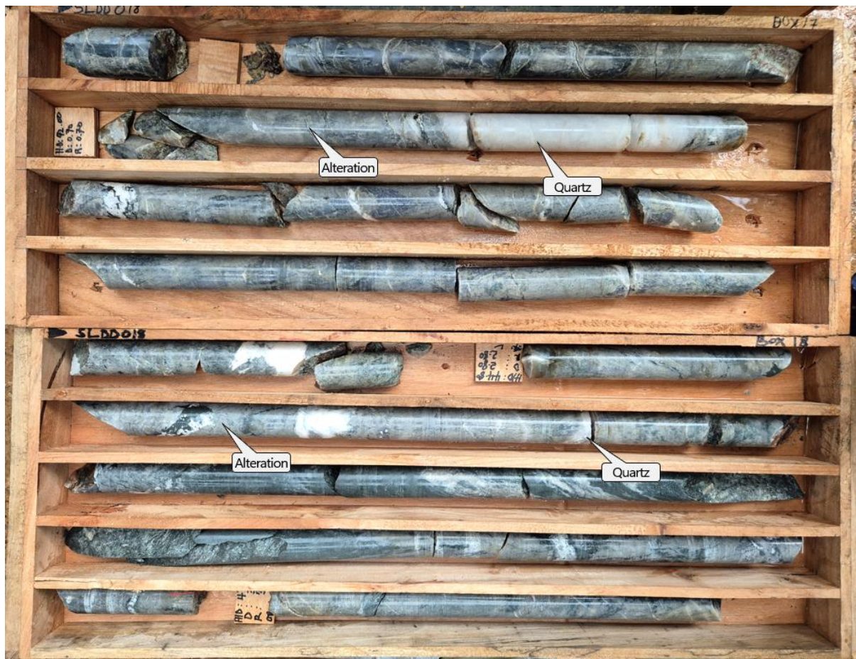
Figure 7: Quartz veining within a broad region of associated brecciation, silicification/chlorite alteration (39.7m to 46m) in SLDD018, interpreted to be the location of the Salanie Fault system (refer Table 2).
