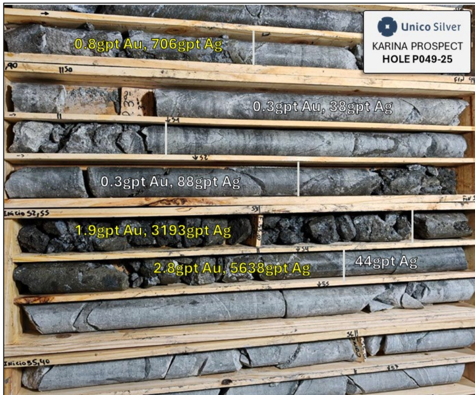
Figure 5: Karina Prospect, hole P049-25 sulphide silver mineralisation
