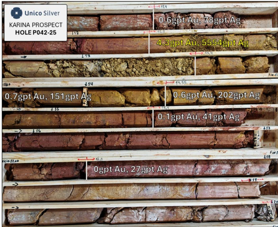
Figure 4: Karina Prospect, hole P042-25 oxide silver mineralisation
