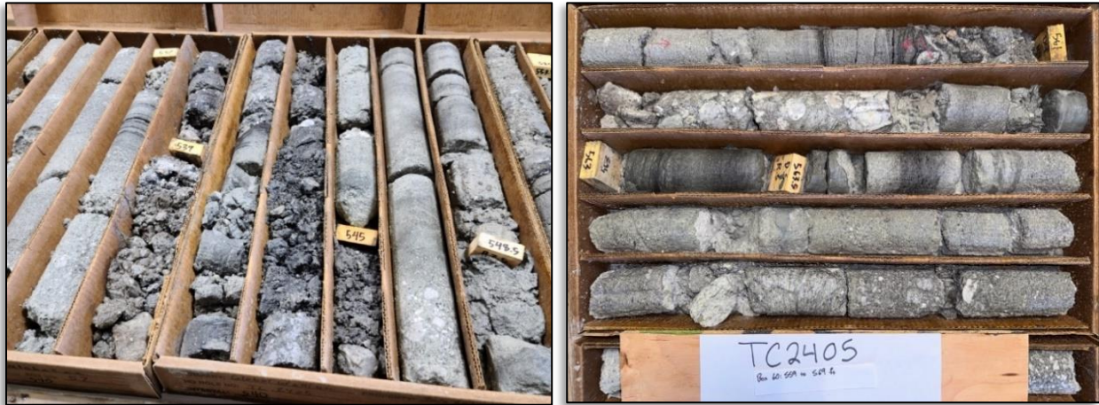
Figure 9: Core from the Project. High Grade 0.562% U_3O_8 drill core from hole TC2405 near 540 ft
