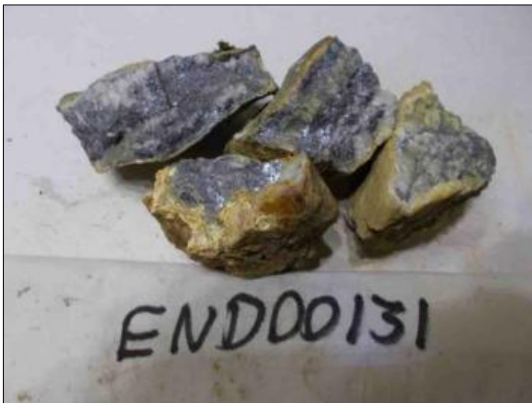
Figure 9. Stibnite bearing ore from the mullock heap below adit No 1 at 440mRL (Green 2015).
