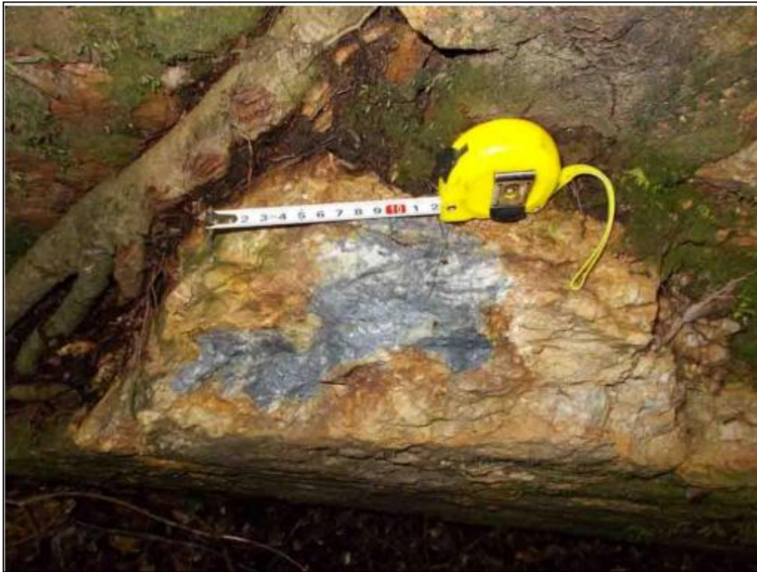
Figure 8. Stibnite-Quartz vein mineralisation remaining in the wall of the Skyline Pit at the uppermost part of the Endeavour Inlet mineralisation (Green 2015).
