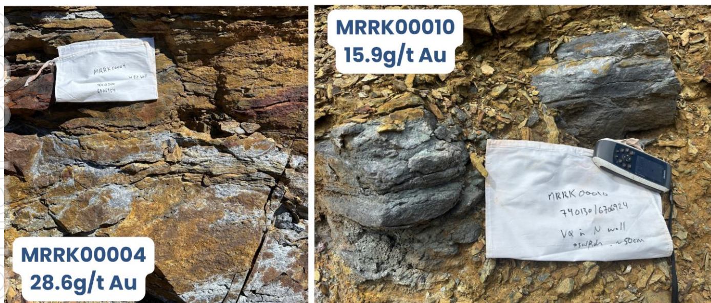
Figure 5 Rock chip samples from pit wall exposures at Evanston Prospect. Left: Sample MRRK00004 (28.6g/t Au), collected from banded iron formation (BIF) with minor quartz and sulphides in the western pit wall. Right: Sample MRRK00010 (15.9g/t Au), collected from a 50cm quartz vein (VQ) with visible sulphides (asp + cpy) in the northern wall.
