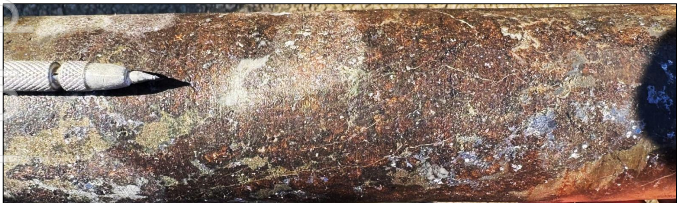
Figure 5: Core photo of skarn-hosted mineralisation with massive sphalerite, galena, chalcopyrite and pyrite from 460.9m in ZRSD25175 – 1.2g/t Au, 0.4% Cu, 2.7% Pb, 8.5% Zn and 60.0g/t Ag (6.7g/t AuEq 2 ).
