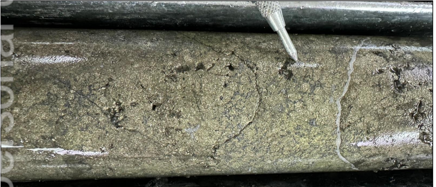
Figure 7: Core photo of skarn-hosted mineralisation with massive chalcopyrite and pyrite from 489.3m in ZRSD25176 – 2.5g/t Au, 1.8% Cu, 0.8% Pb, 0.2% Zn and 35.2g/t Ag (5.6g/t AuEq 2 ).
