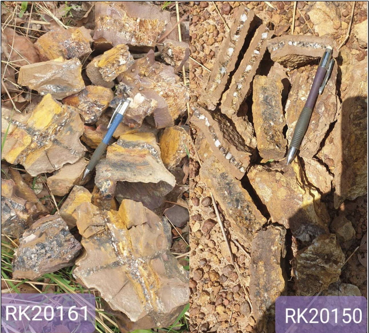
Figure. 6: Photographs of rocks collected/observed at Timbakouna with quartz veined metasedimentary rocks noted over extensive areas. Reported here are sample RK20161 which did not return a significant gold result (<0.01 g/t) and sample RK20150 returned a gold result of 2.92 g/t – see Table 3 and 4.
