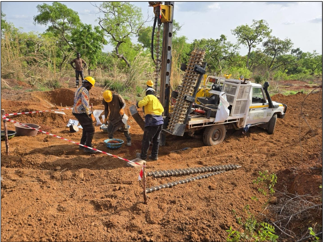
Figure 1 – Power auger drilling being completed at the Dadjan Gold Project, located in the Siguiri Basin, Guinea.
