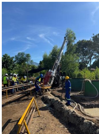
Figure 2 Diamond drill rig in operation
