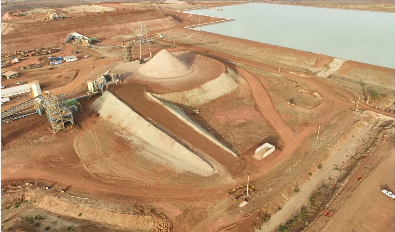
Photo 4: Kiaka coarse ore stockpile with ROM pad and water storage facility in background
