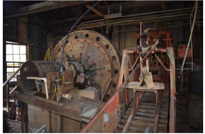
Photo 2. Ball mill within the mill building.
