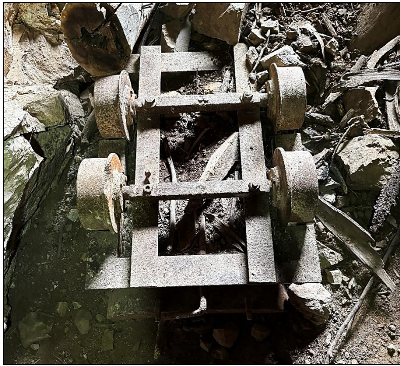
Photo 3. Magwood mine ore cart. Primitive historical mining methods resulted in only the highest-grade antimony mineralisation being mined and hand sorted
