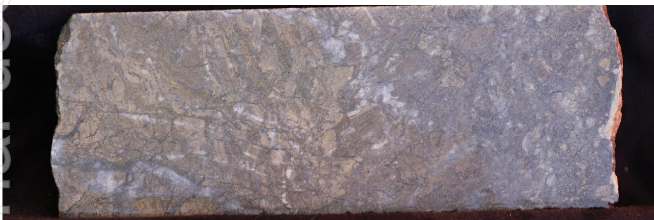
Figure 7 NSD058, 283.65m, fine-grained, acicular (needle-like) arsenopyrite in brecciated sulphide.
