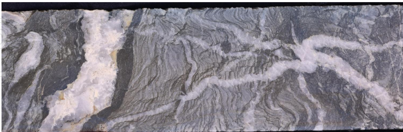
Figure 5 NSD058, mineralised upper contact of interpreted basalt.
