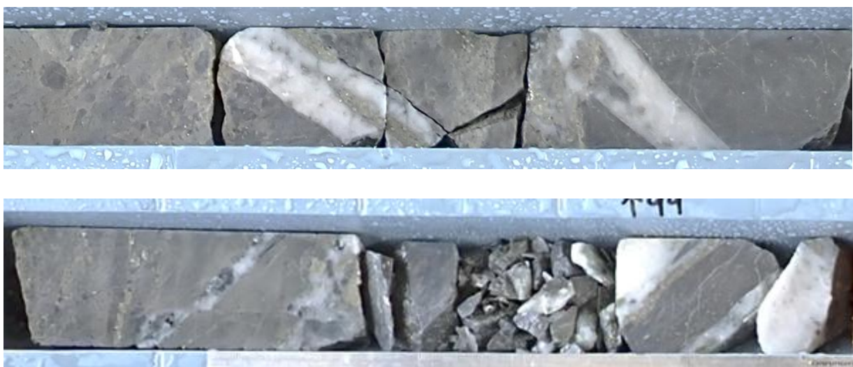
Figure 5 – Examples of the Displaced Lode including quartz-pyrite-chalcopyrite veining in sericite-altered volcanic in DTDD054 (99.3 – 99.6m & 99.6 – 100.0m).
