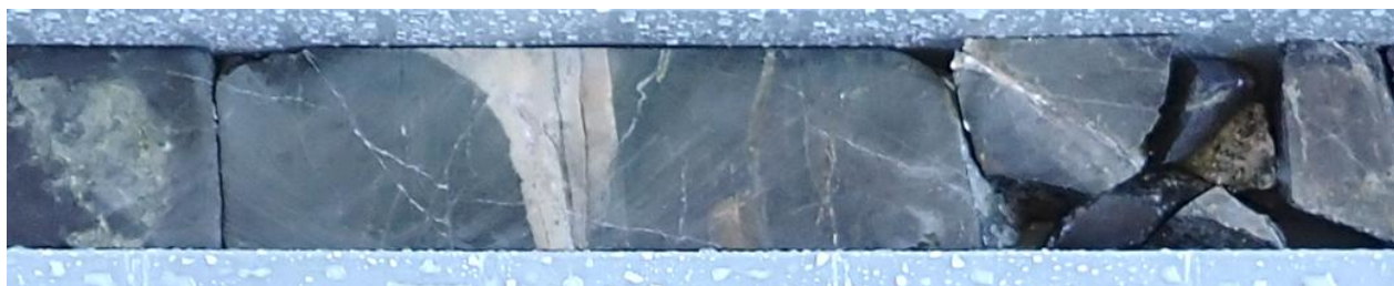
Figure 2 – Examples of 1-3cm wide Quartz-carbonate-pyrite vein at 158.2 – 158.5 in DTDD052
