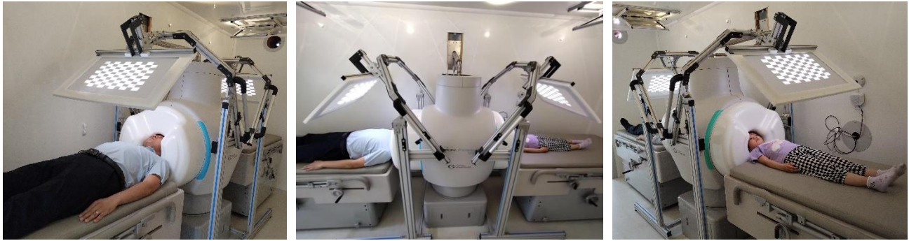
Orion LifeSpan™ configured for hyperscanning. Father and daughter subjects are measured simultaneously to study interactions. Synchronisation of the sensors in the two helmets is within 1 msec. Pic: Compumedics
