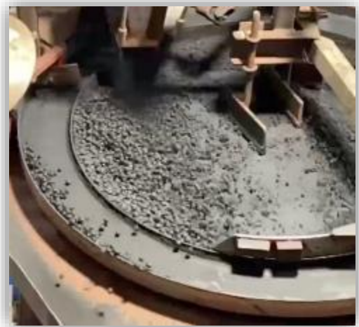
Picture 2. Green Ball manufacture in pelletising disc
