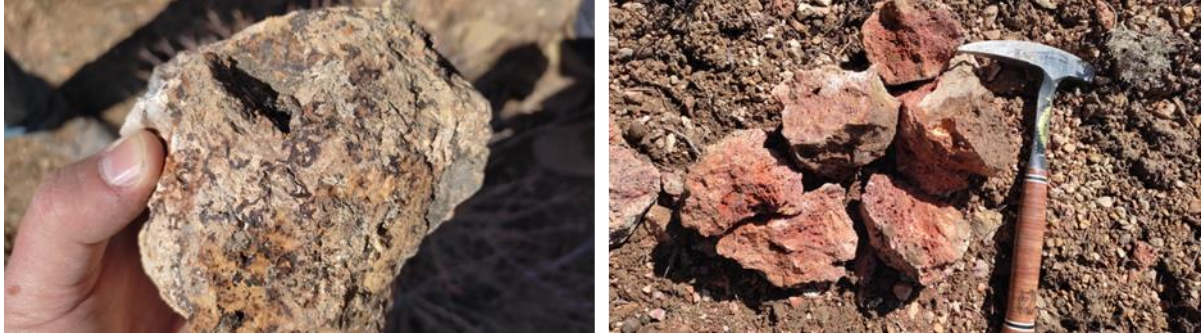
Figure 7: Bayan Springs South Samples - Intensively Silicified and Oxidised Breccia Samples 190036 (left) and 19037 (right)
