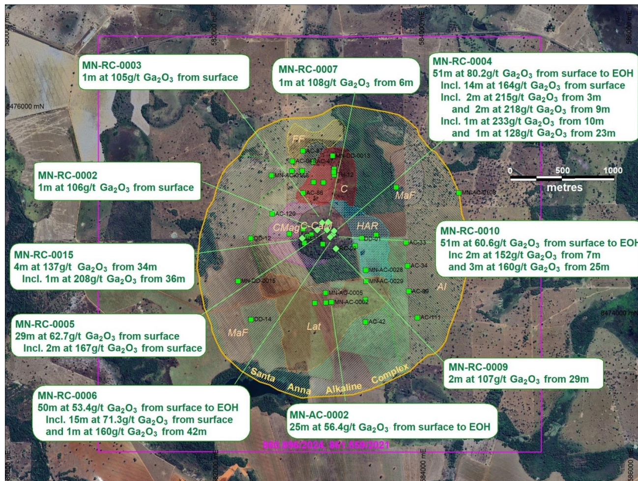
All drillholes containing at least one sample with 50g/t Ga 2 O 3 or greater is show as green dots
