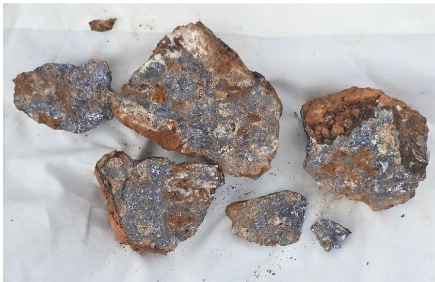
Figure 1: Altered vein sample THRK023 taken from Thowagee historical working returned 12.2% Pb, 170g/t Ag, 0.7% Zn.
