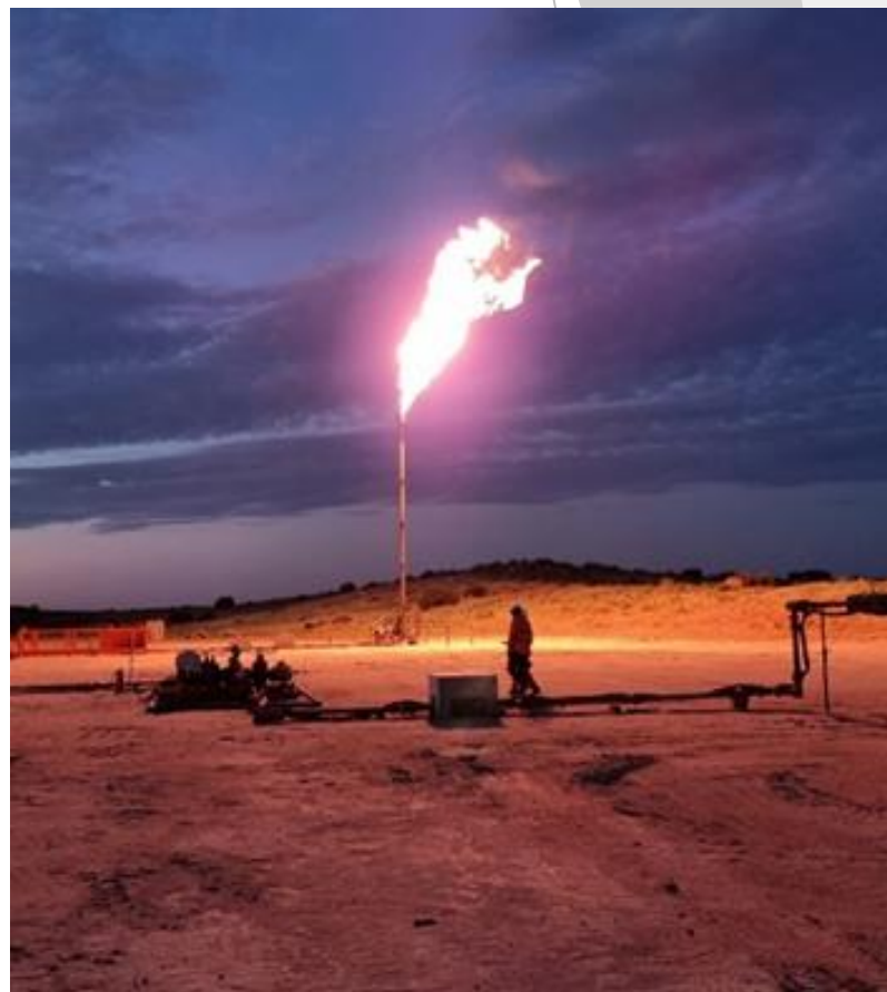
Figure 1: Gas flare from Kiwi-1 wellsite at 1.7 mmcf/d
