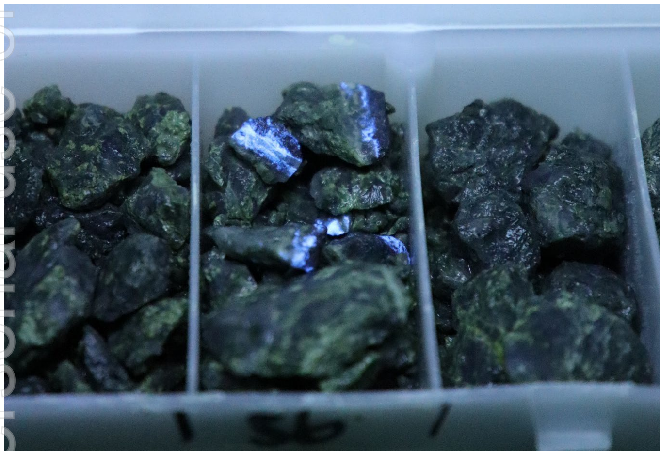
Figure 2: Scheelite mineralisation (bright light blue) observed in RC drill chip from Clarks Gully samples under UV light. CLG078 73-74m depth; assayed at 0.27% WO_3
